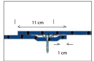
Spacing between the disc and membrane overlap should be 11 cm.
