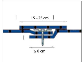
b) This system is also used in lightweight roof construction to form the edge and corner regions in the longitudinal direction of the corrugations. The fasteners are arranged as prescribed along the laid membrane and covered with 15-25 cm wide strips of material.
