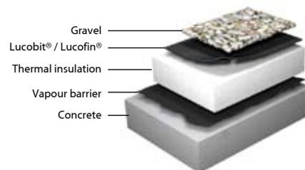
Roof structure with gravel ballast
