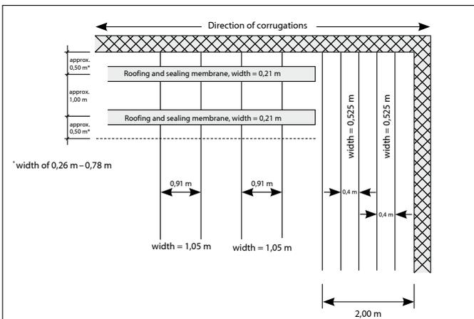
Sample diagram for laying Lucobit® / Lucofin®. Other sample diagrams are available upon request.
