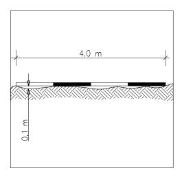
Out-of-plane under a 4 m rod: maximum 10 cm
