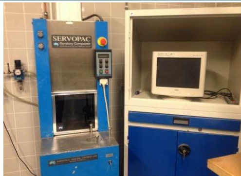
Compaction Until the Hight of sample reach 150 mm
