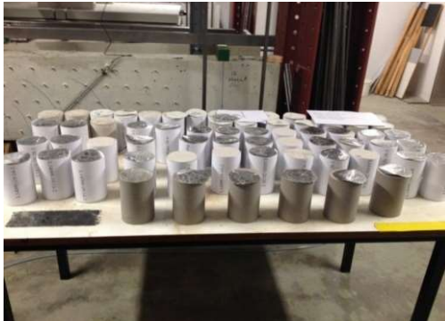
Sample Diameter: 100 mm Height: 150 mm
