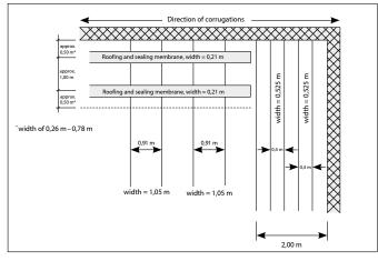
Sample diagram for laying Lucobit<sup>®</sup> / Lucofin<sup>®</sup>. Other sample diagrams are available upon request.
